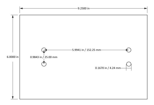
Board mounting holes are spaced to be used with DIN rail clips. Otherwise, standoffs can be mounted and used if preferred.
